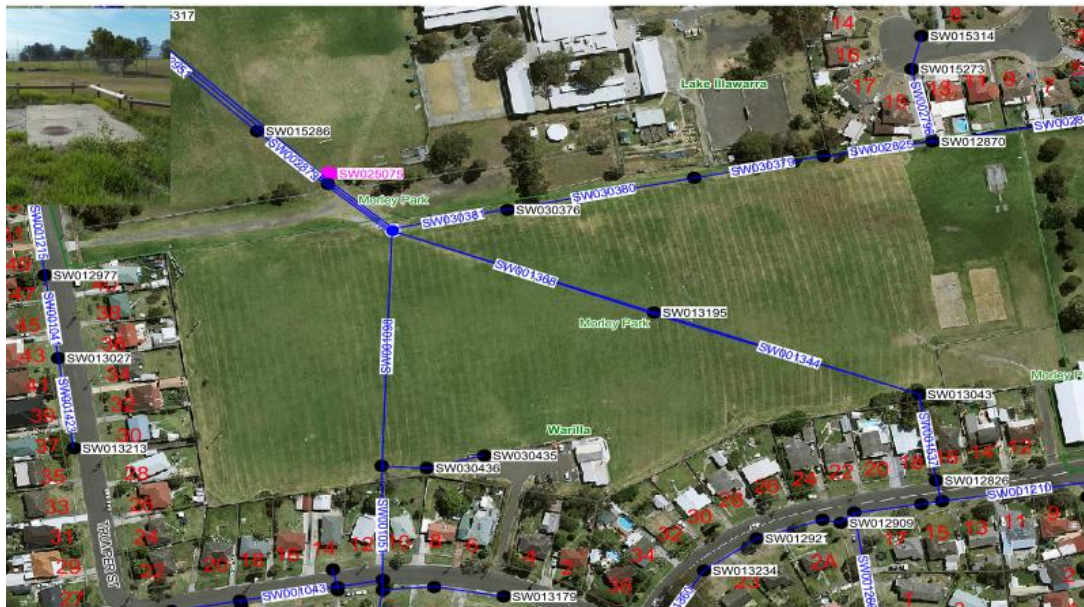
Figure 4 - Storm water plan, Morley Park. Inset (top LHS) Junction Pit.
